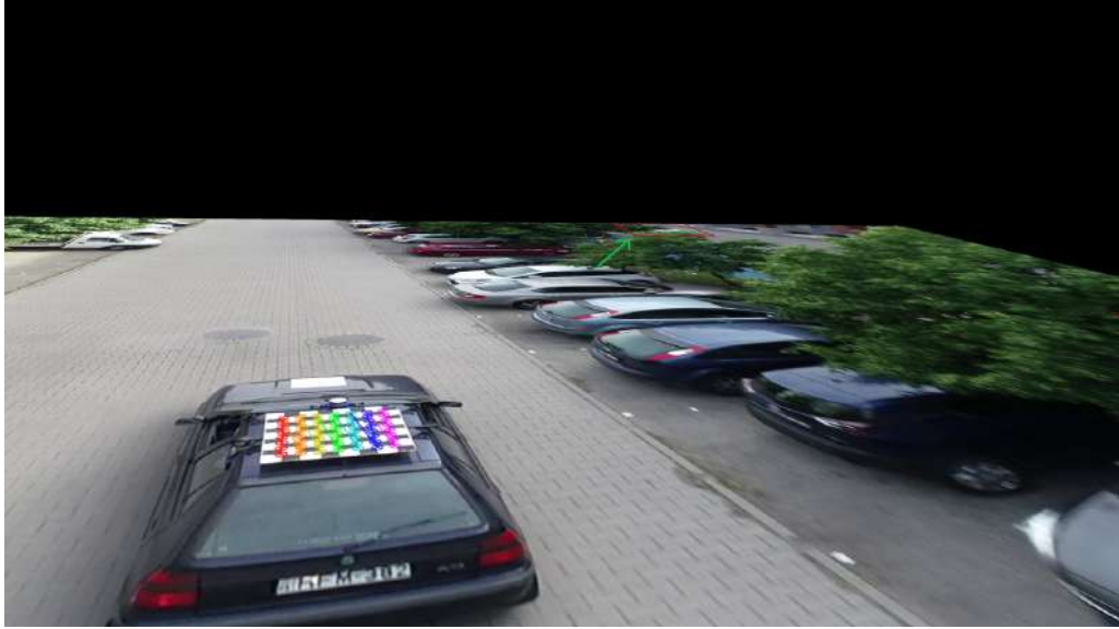
Figure 3.29: Perspective transformation showed the car's location (green arrow).
