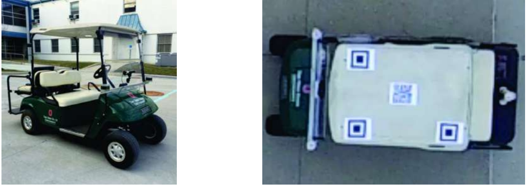
Figure 1.2: EZ Golf Cart as vehicle agent (left) and the markers on top of the car (right).[3]
