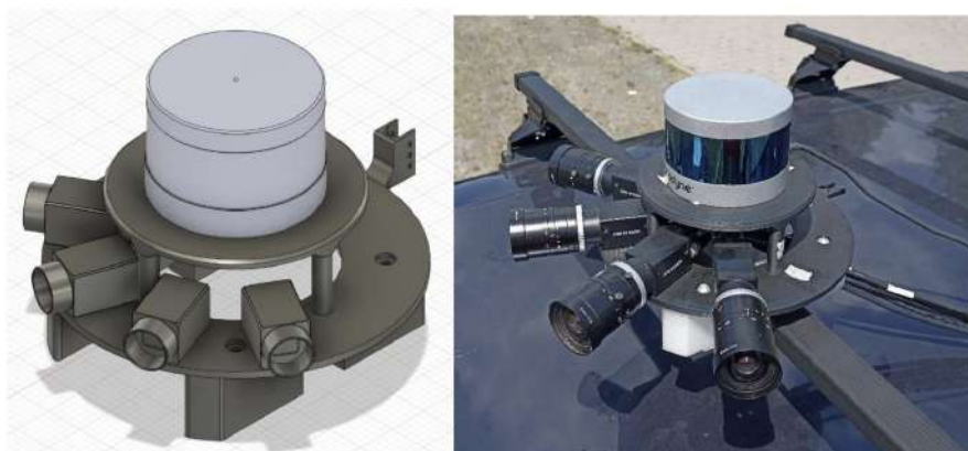
Figure 2.15: ELTE Car Camera Installation
