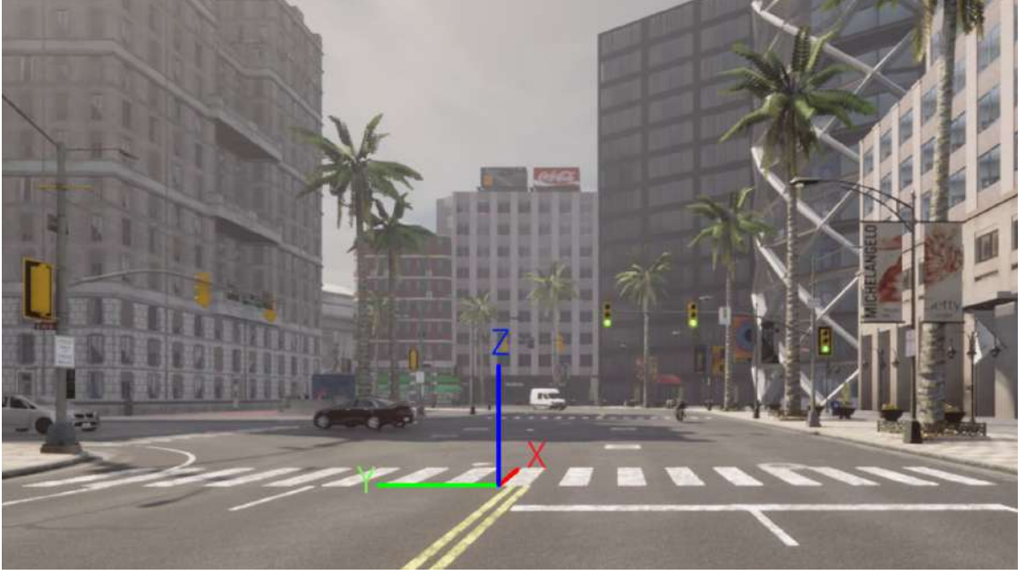
Figure 3.7: The coordinate system on the road plane.
