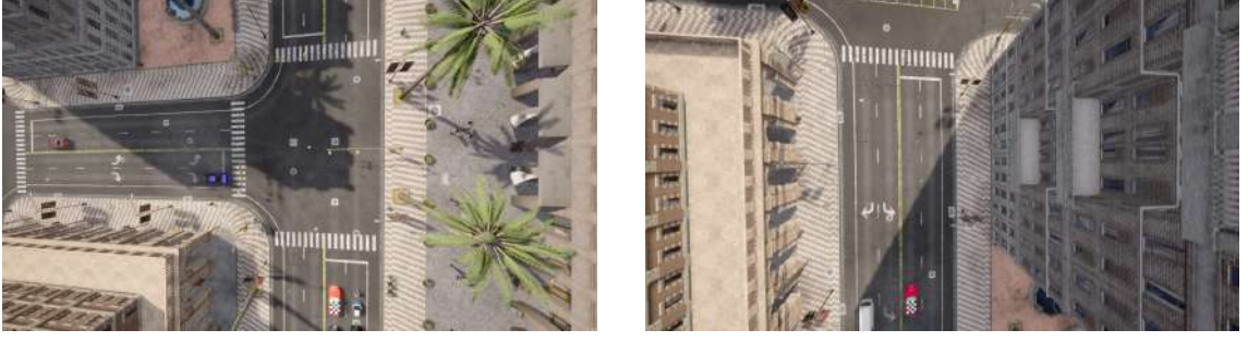
Figure 2.13: Rotation effect on a drone-mounted camera positioned at 35 meters height.
