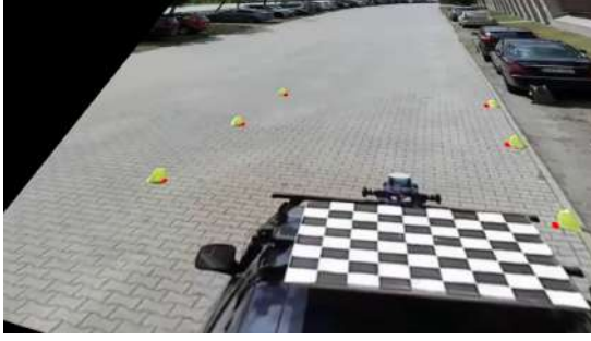
(b) Projective transformation from the drone-mounted camera's image.
