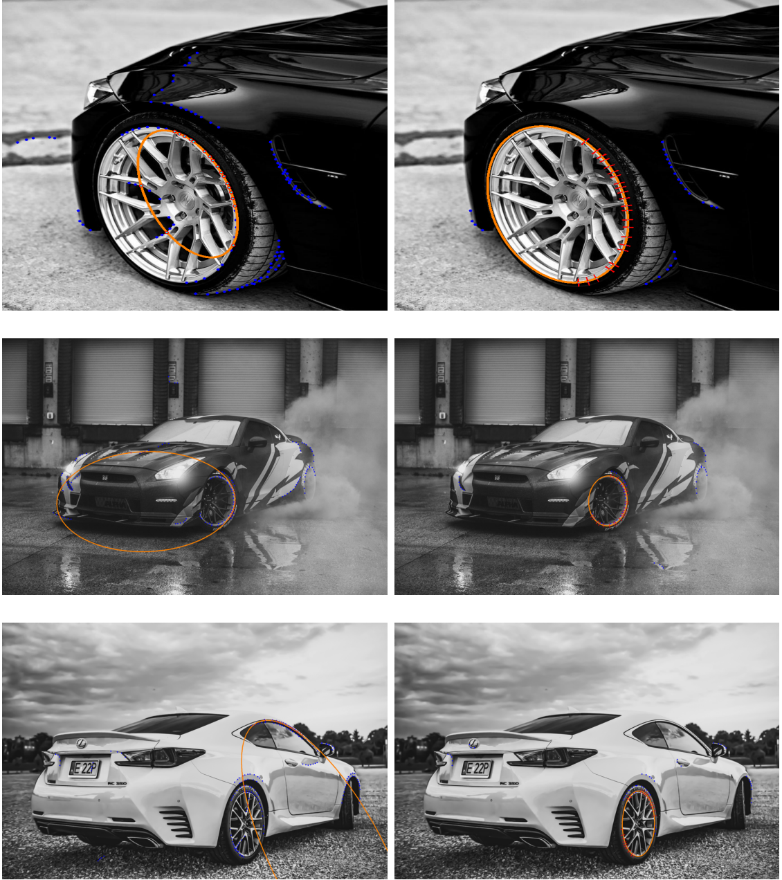
Figure 5.9: Good results fitted by oriented ellipse fitting on wheel images(right) and corresponding results of direct ellipse fitting(left). There's no indicate points for center estimation since the images are taken by unknown cameras.
