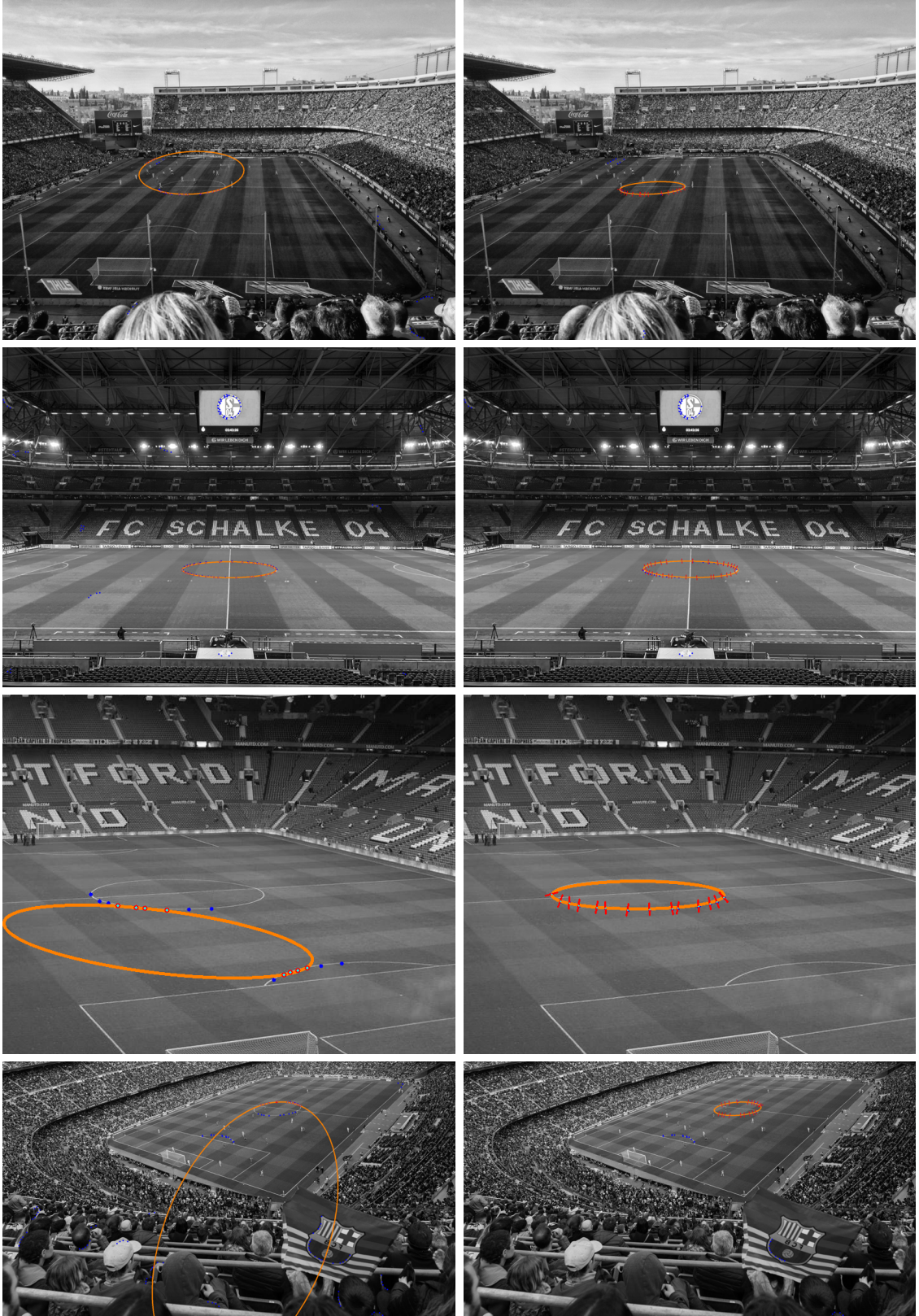
Figure 5.11: Good results fitted by oriented ellipse fitting on soccer field images(right) and corresponding results of direct ellipse fitting(left).
