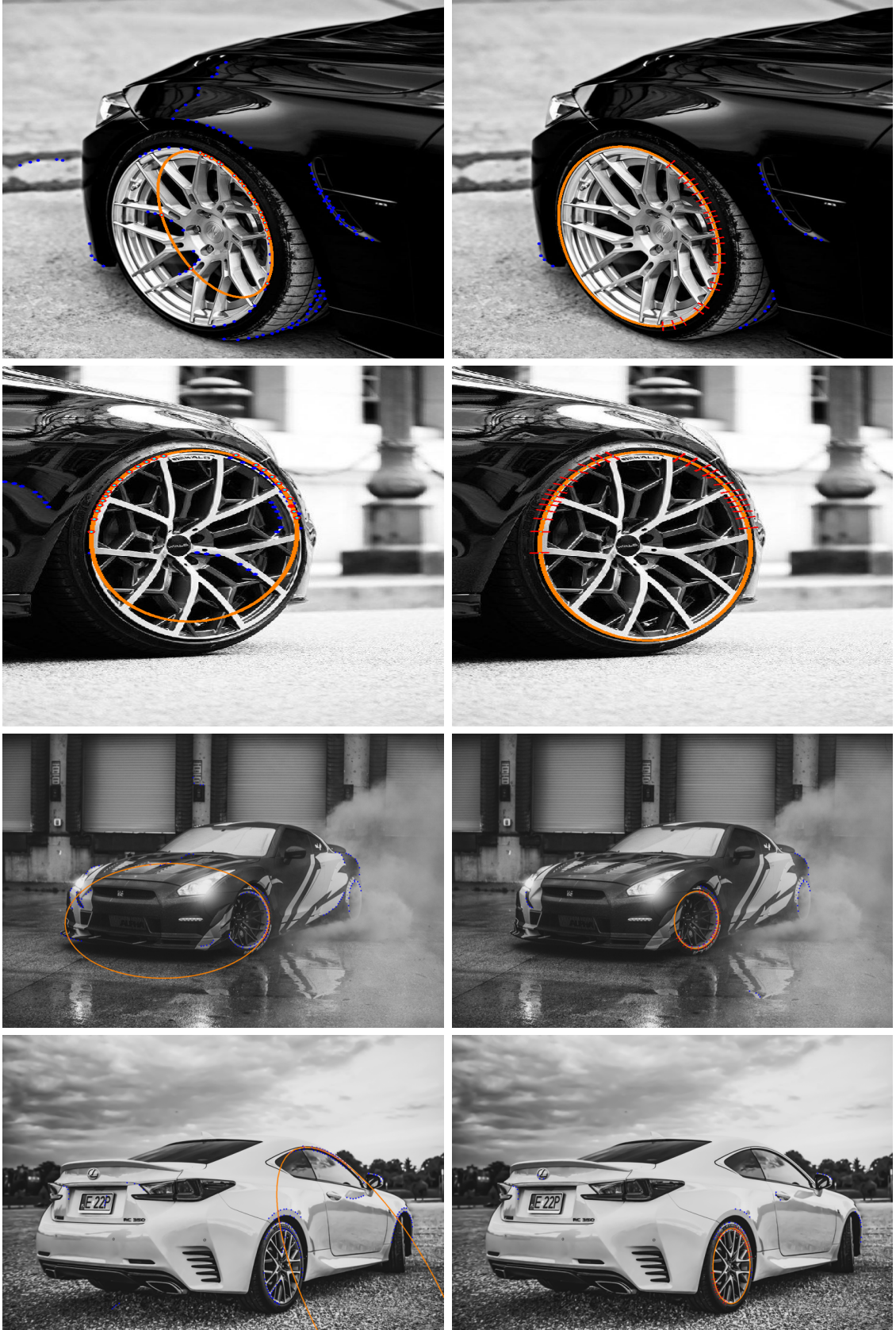
Figure 5.9: Good results fitted by oriented ellipse fitting on wheel images(right) and corresponding results of direct ellipse fitting(left). There's no indicate points for center estimation since the images are taken by unknown cameras.
