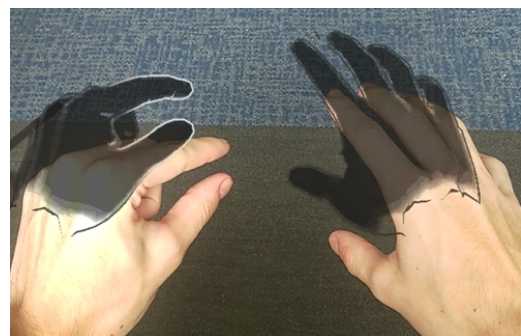
(b) The generated hand mesh overlaid the real hand. The left-hand uses a pinch gesture. The recognition of this is indicated by the white outline of the two fingers.
