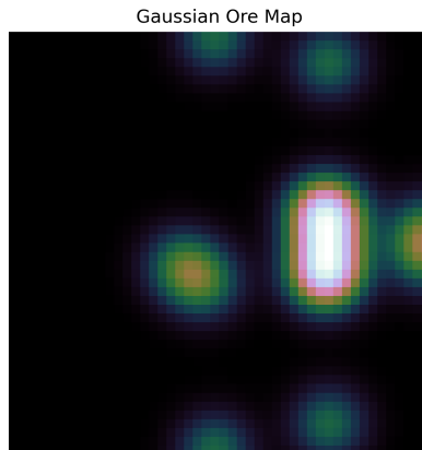
Figure 2.8: High presence of ore calculated using our Gaussian filter. Lighter values indicate high-density ore areas.
