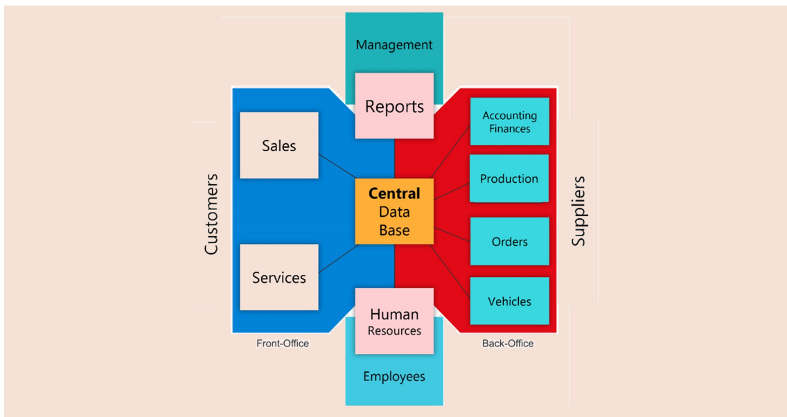
Figure 2.3: Anatomy of an Enterprise System (adapted from [19]).
