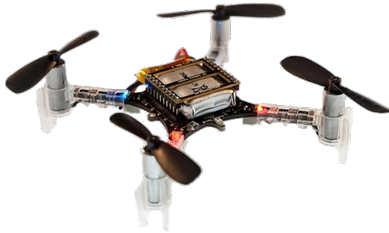
Figure 3.1: The Crazyflie 2.0 miniature quadrotor.
