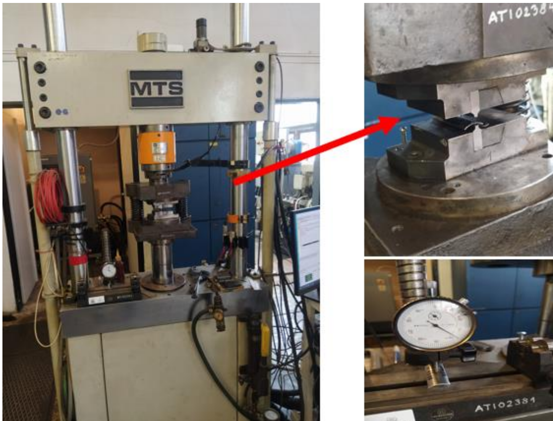
Figure 6: MTS operations and data recording for material characterization
