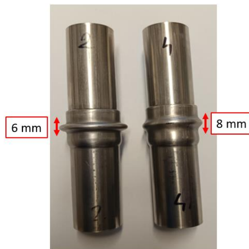
Figure 17: Joints of 6 mm and 8 mm thickness formed at 50 mm die gap distance
