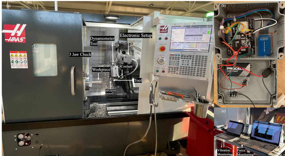
Figure 7. (a) HAAS ST-20 Y CNC Machine (b) Electronic setup (c) Real time monitoring vibration and cutting forces
