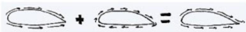
Figure 29 Resultant of Air Flow and Circulation[33]
