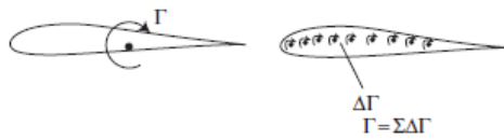
Figure 31 Vorticity Concentrated on the Camber Line [32]
