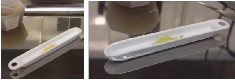
Figure 9: Left: before annealing, little grains of perovskite was visible in the mixture resulting in the darker orange color. Right: after annealing, the grains disappeared and the sample became yellow.
