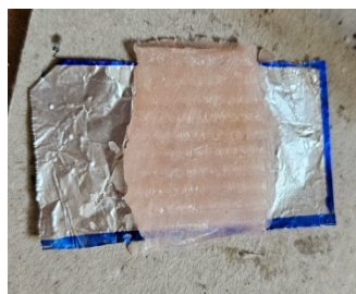
Figure 4. (b) Initial layer of wax on aluminum foil
