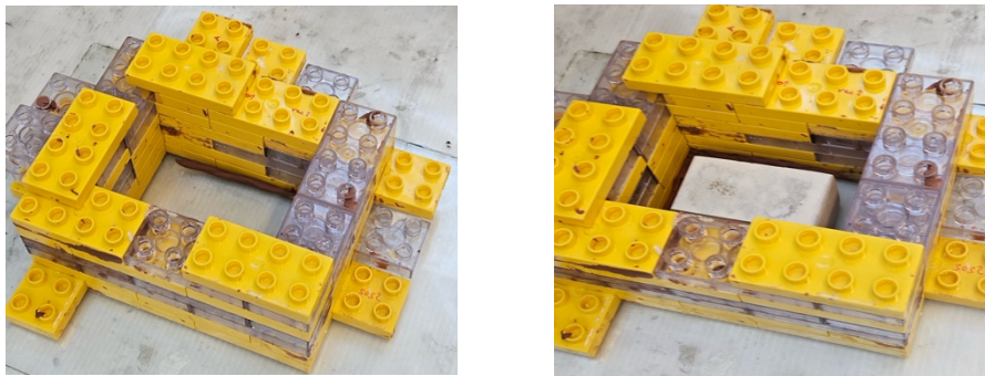
Figure 6. (c, d) Block construction for silicon casting with 20 mm space around the gypsum in all directions
