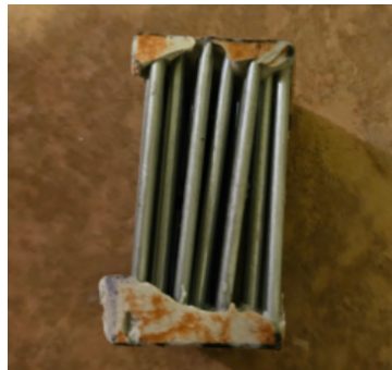
Figure 16. Skewed tube arrangement
