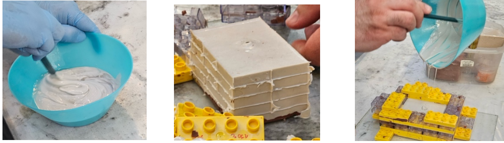
Figure 6. (e) Mixing of silicon with silicon catalyst (f) Hardened silicon mold (g) Pouring of earlier mixture into block construction
