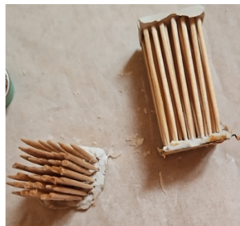
Figure 5. (b) Tube arrangement secured with gypsum after wax was burned out. Bottom left is fixed only on one side while top right is fixed on both ends modelled with toothpicks.
