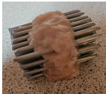
Figure 4. (d) Tube arrangement bound by paraffin wax
