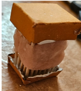
Figure 5. (a) Tube arrangement bound by paraffin wax and fixed with gypsum
