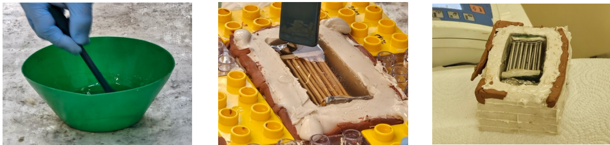
Figure 6. (h) Epoxy mixture (i, j) Tube arrangement infiltrated with epoxy
