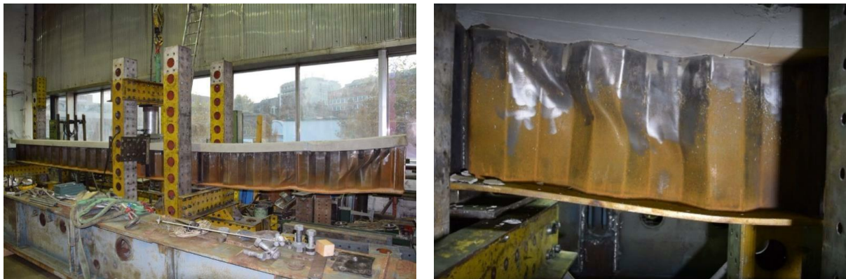
6.7. Figure: B-1-3 initial setup and deformed CSW
