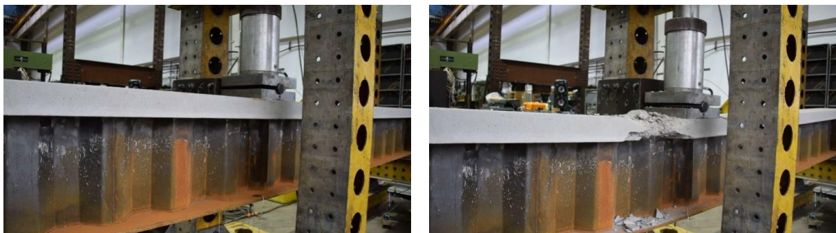
6.10. Figure: B-4 undeformed shape and failure mode
