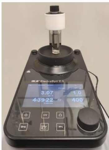
Scheme 15. IKA ElectraSyn 2.0 Package used for electrocatalytic oxidation of amines.
