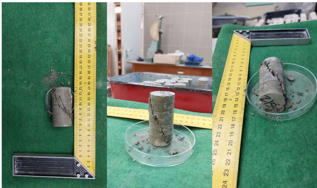
Figure 22: Examples of samples after UCS test
