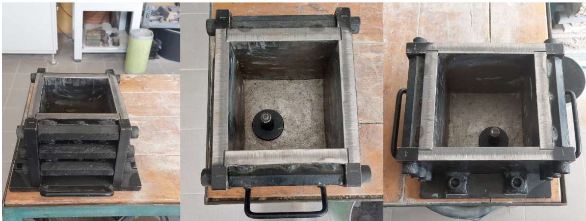
Figure 8: Mould used for cubic samples
