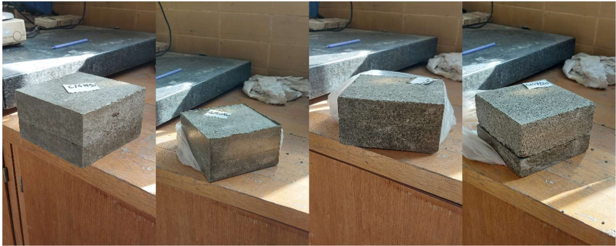
Figure 20: Cubic samples with visible inhomogeneous
