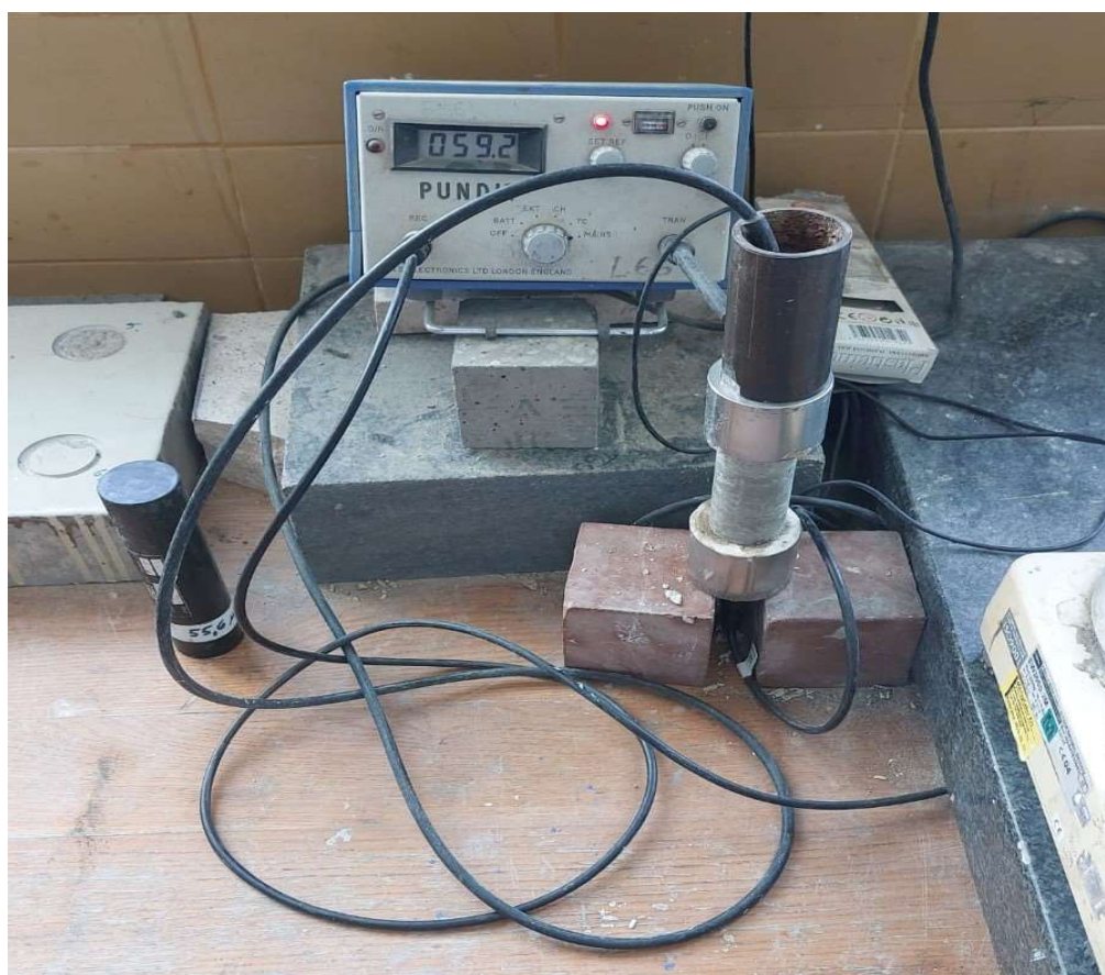
Figure 17: Ultrasonic machine used for the UPV testing. Cylindrical sample can be seen between two transducers
