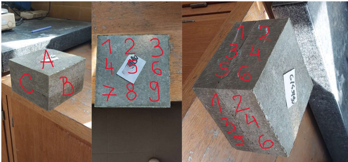
Figure 18: Cubic samples and points for the UPV test.
