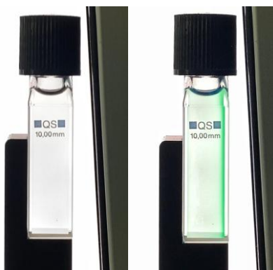
Figure 34. Color change of the modified reversible photoswitch ( 7 ) upon irradiation with 312 nm light.
