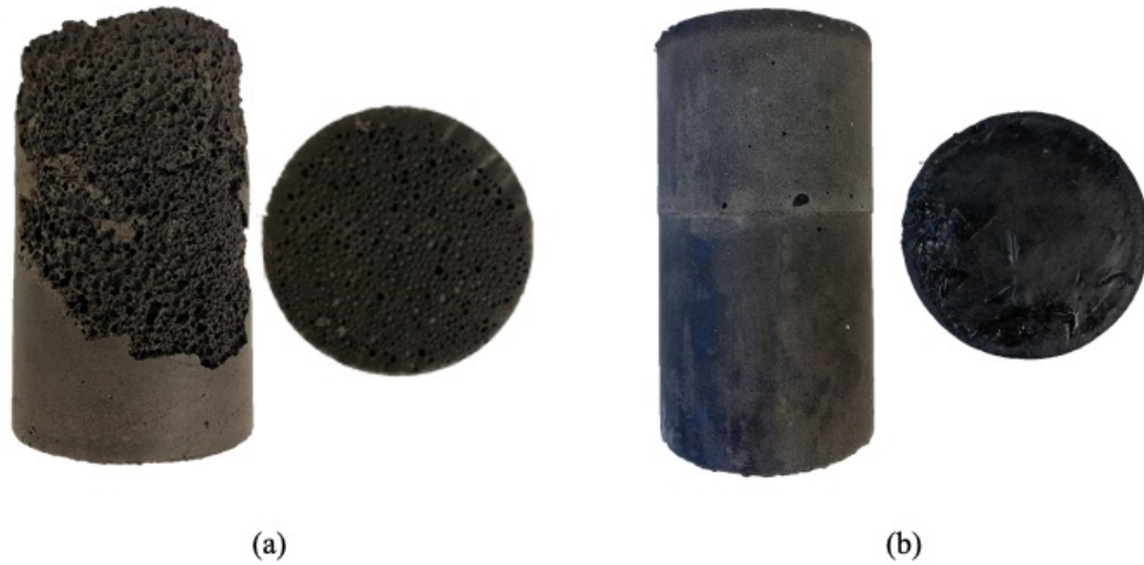
Figure 19. Geopolymer specimens after aging 7 days. (a) Foamed Geopolymer & (b) Non-foamed Geopolymer.
