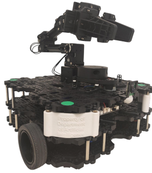
Figure 3.10: TurtleBot3 Waffle Pi with OpenManipulator-X
