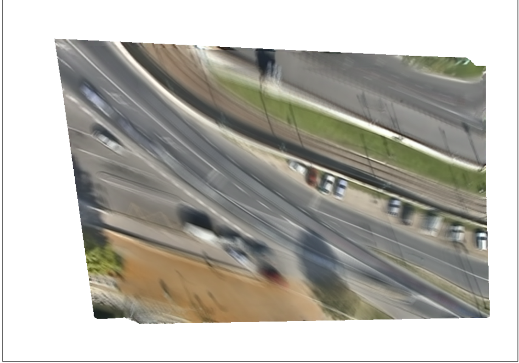
FIGURE 2.4 Average of 100 frames when image registration uses only pairs of consecutive frames. Compare with Figure 2.5.
