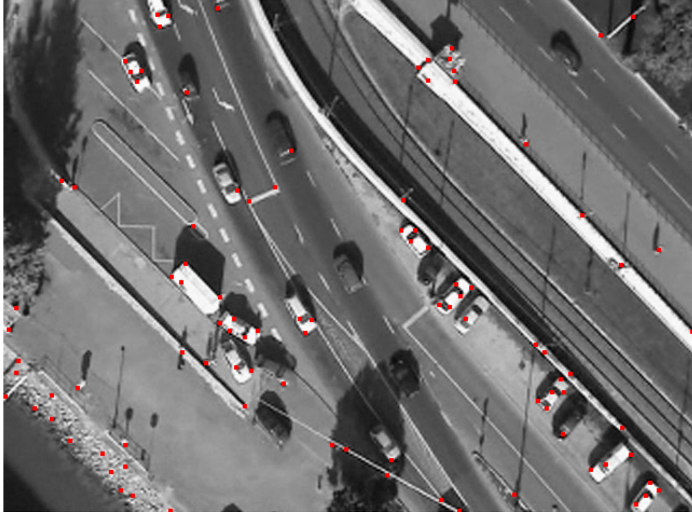
FIGURE 2.2 Feature points of a grayscale image found by Harris corner detector.
