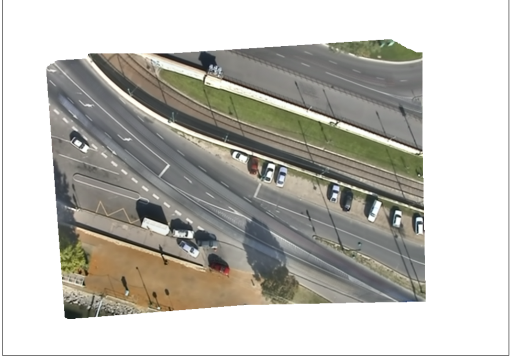
FIGURE 2.5 Average of 100 frames when frames are registered against the background image. Compare with Figure 2.4.
