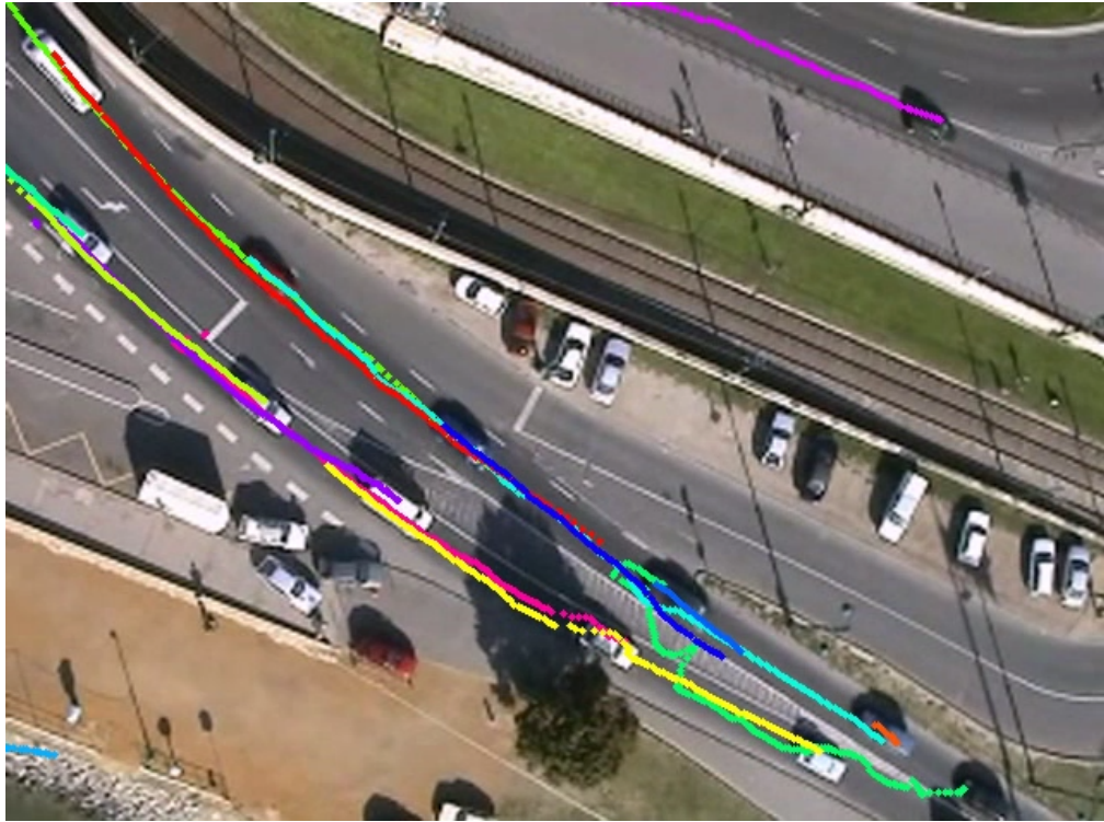
FIGURE 3.1 Detected tracks with different hue. Erroneous detection in cyan is seen at the bottom left corner. Confused track is visible in light green at the bottom right corner. This example is from a real urban scene.
