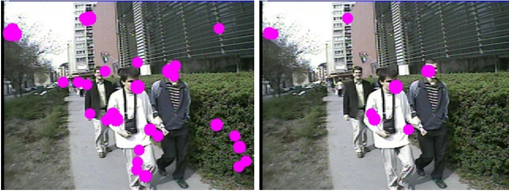
Figure 6.4: Comparison of the fixation patterns on images with and without filtering. The left image shows the generated output where estimated points are located at the periphery of the images as well. The right image is after filtering the less probably attractive fixation points according to HVS-based statistics.
