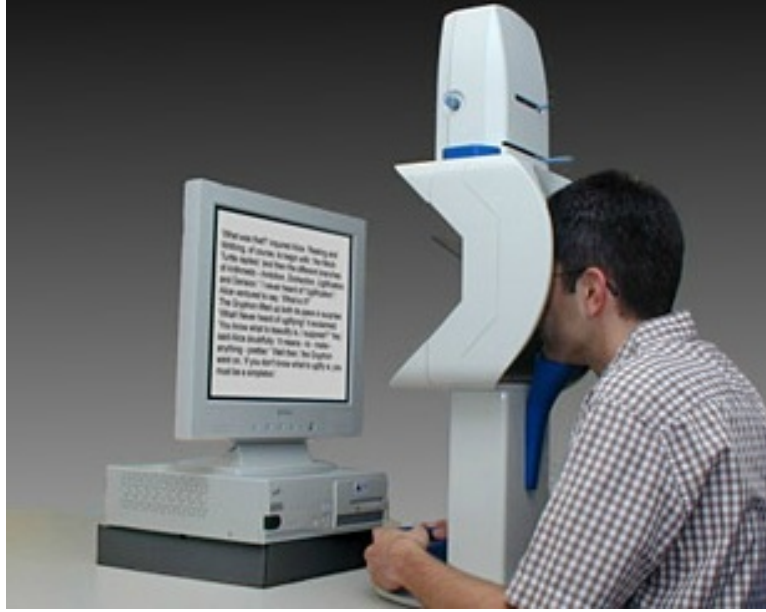
Figure 6.1: iView X fast, accurate, video-based eye tracker. Volunteers using this device were taking part at verification experiments. Some images were displayed in blocks in a large monitor, and the observers were asked to memorize the images. The recorded human eye movement was then compared to the estimated Regions-of-Interest inferred by our model.
