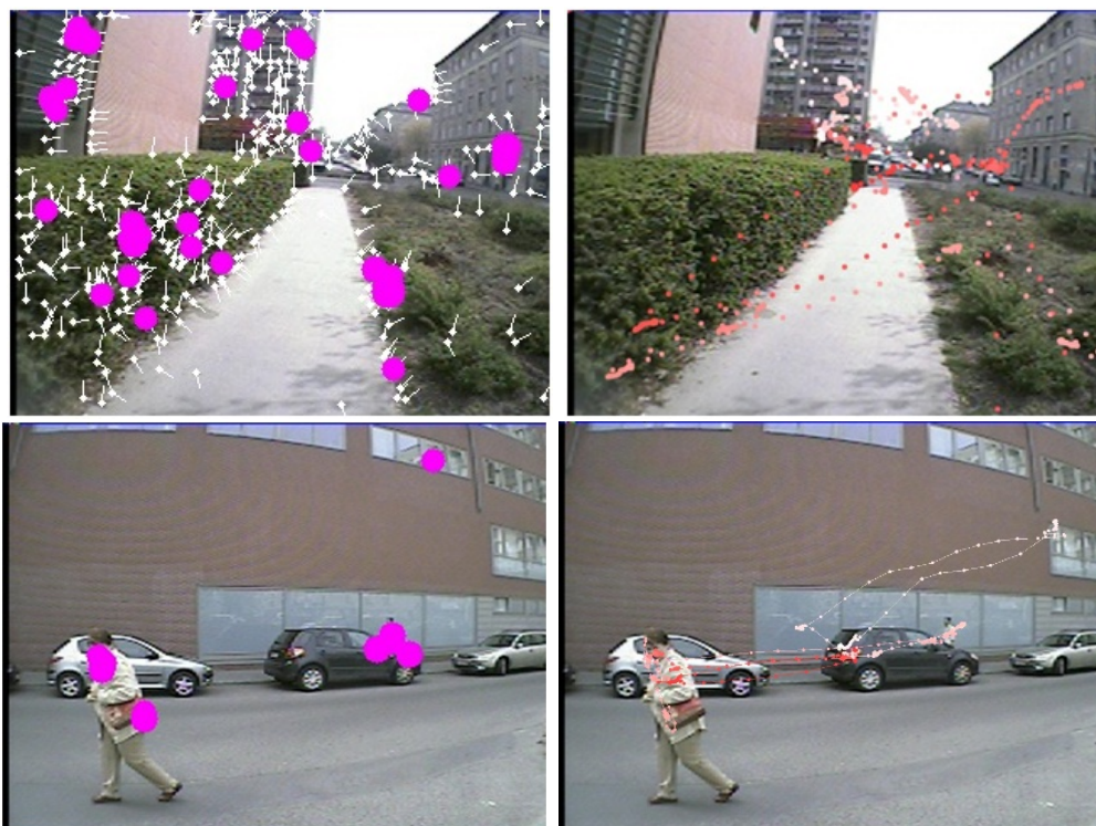
Figure 5.3: Comparison of the most probable gaze points to the real human gaze path. Images on the left images show the estimated points based on the transition probability graphs with statistical summary, which were trained by evaluating some other videos. For verification, images on the right show a real human eye movement of the same images.
