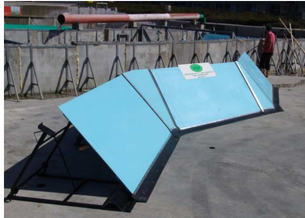
Pic. 26: The triangular dykes are very flexible in point of placement
