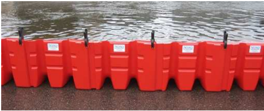
Pic. 30: Butterfly dyke can't prevent leakage even on a demonstration...
