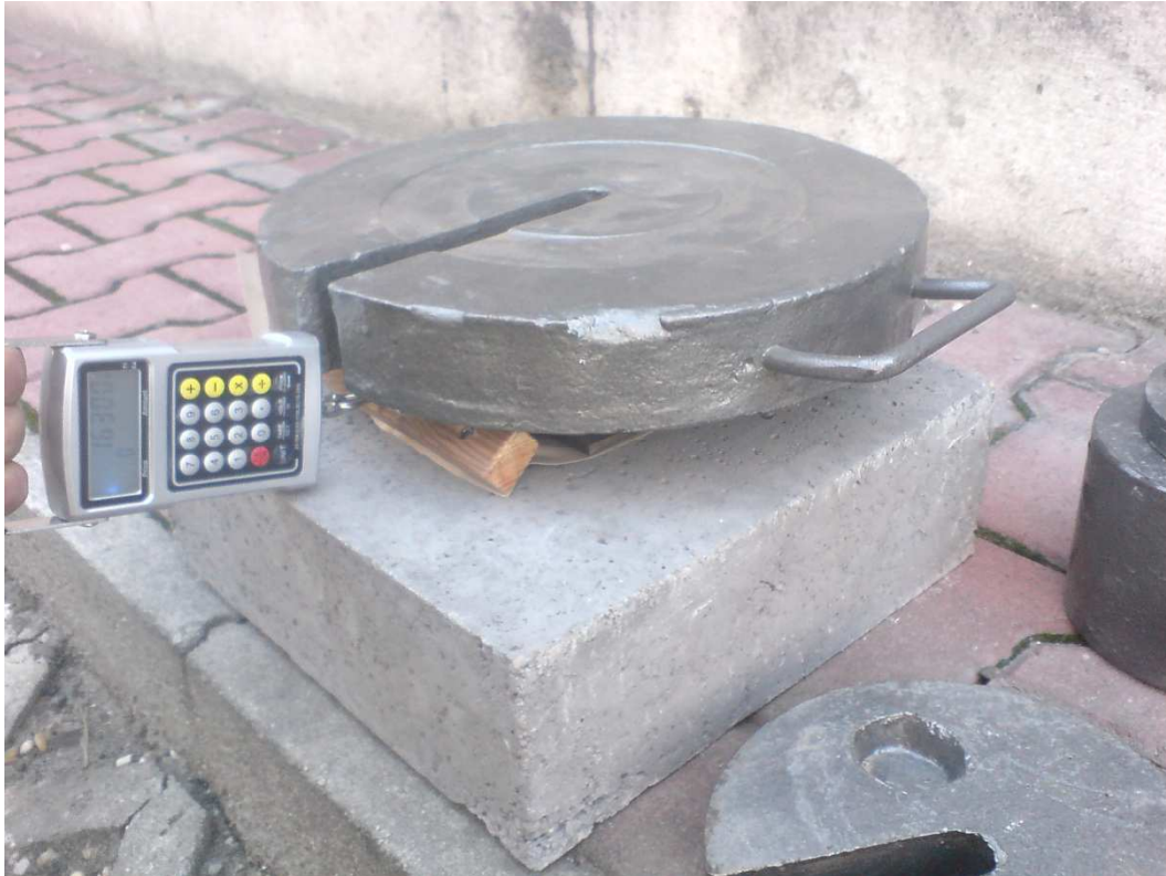
Pic. 43: Field test on a concrete prism
