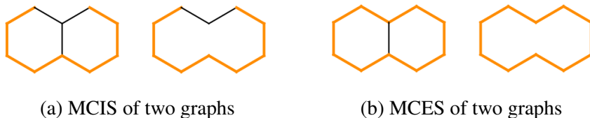
Figure 1: An example of the difference between the MCIS and MCES of two graphs
