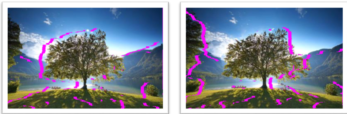
Figure 20: Stereoscopic left and right images with blank pixels ( maxParallax at 16 pixels)
