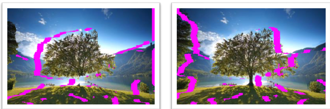
Figure 21: Stereoscopic left and right images with blank pixels ( maxParallax at 32 pixels)
