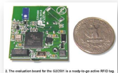
2. The evaluation board for the G2C501 is a ready-to-go active RFID tag.
