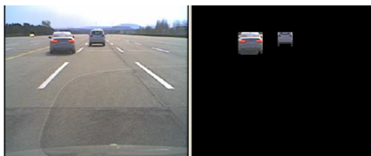
Figure 2.2: Road segmentation by shadow-like features. After shadows are found on the input images (left) the areas above them are processed (right). Source: [3]
