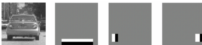
Figure 2.4: Examples for the patterns implemented by Haar-like features. The first pattern validates the existence of a shadow below the car while the other two match the wheels. Source: [2]
