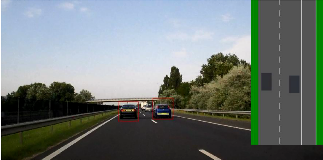
Figure 5.3: Sample image to demonstrate the efficiency of the detection based overview. Both car are recognised, tracked and positioned in the projected 2D space. Also, license plates(5.3) are detected and marked with yellow.
