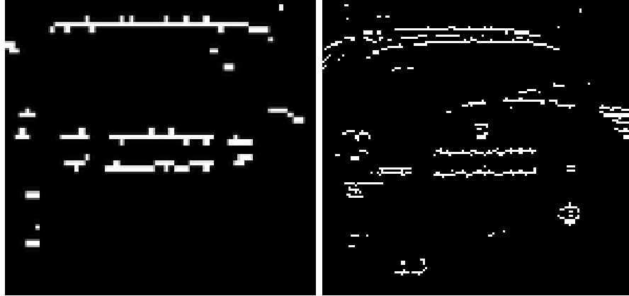
Figure 4.6: To detect the license-plates, horizontal edge-maps are used. Notice the strong outlines of the plates. Strongest horizontal edges are chosen during the process. Each gap between neighboring is analysed. The algorithm searches for a bright, rectangle-shaped object. See section 5.3 for results.
