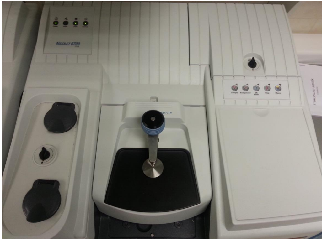
Figure 1; Thermo Scientific NICOLET 6700 FT-IR infrared wavelength spectroscope
