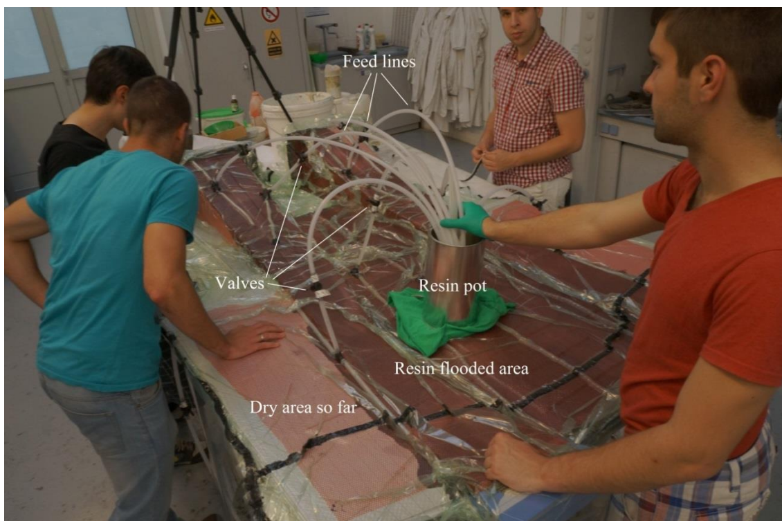
Figure 152: Resin transfer
