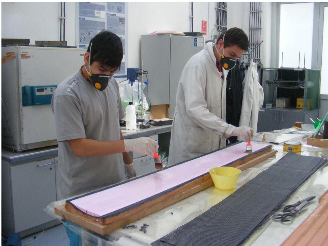
Figure 155: Resin application by hand
