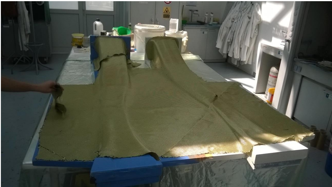
Figure 146: Aramid-Carbon fibre layer created of several pieces
