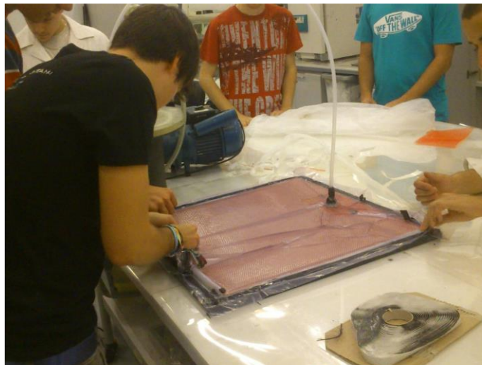
Figure 83: Preparations for the vacuum infusion
