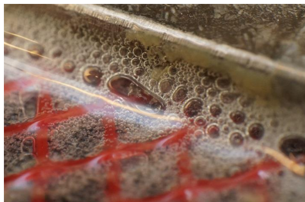
Figure 151: Air bubbles in the resin
