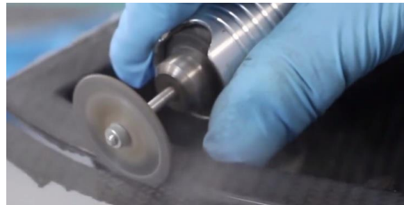
Figure 159: Cutting with Dremel
