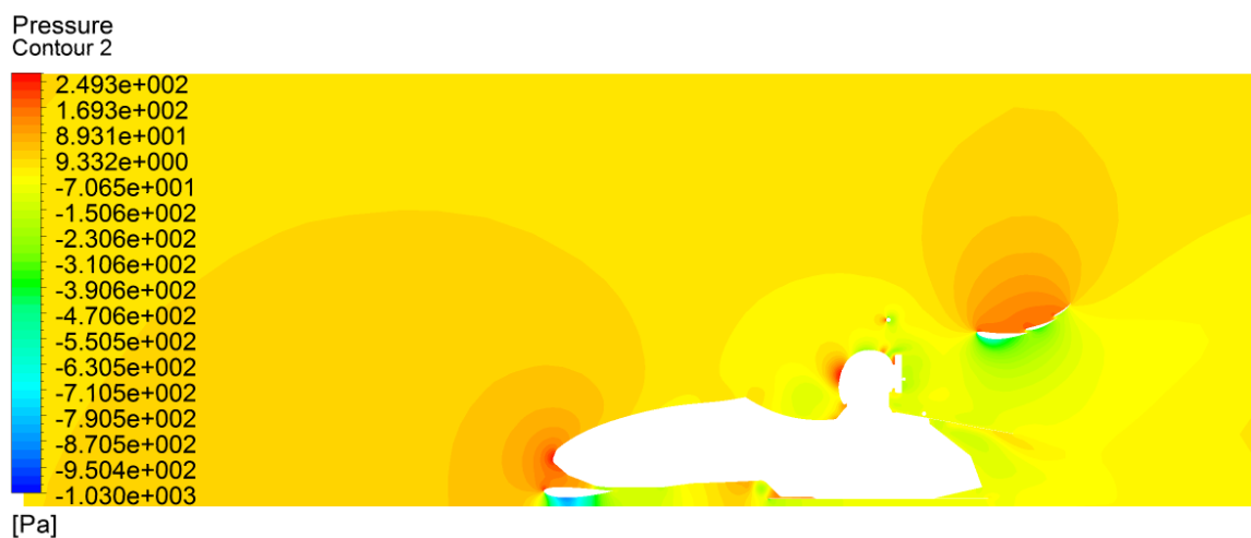
Figure 55: The pressure distribution on the symmetry plane
