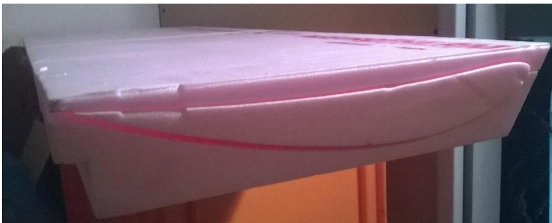
Figure 141: Foam moulds with foam core
