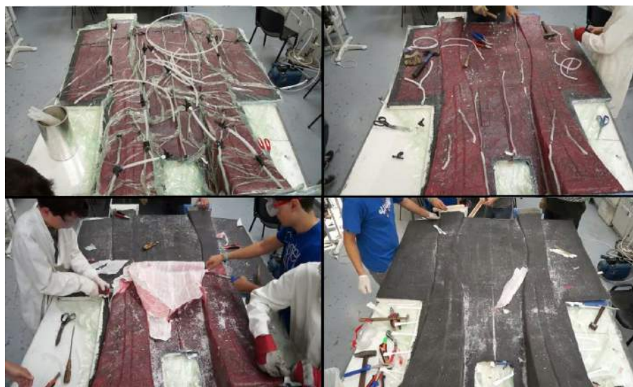
Figure 156: Removal of the auxiliary materials
