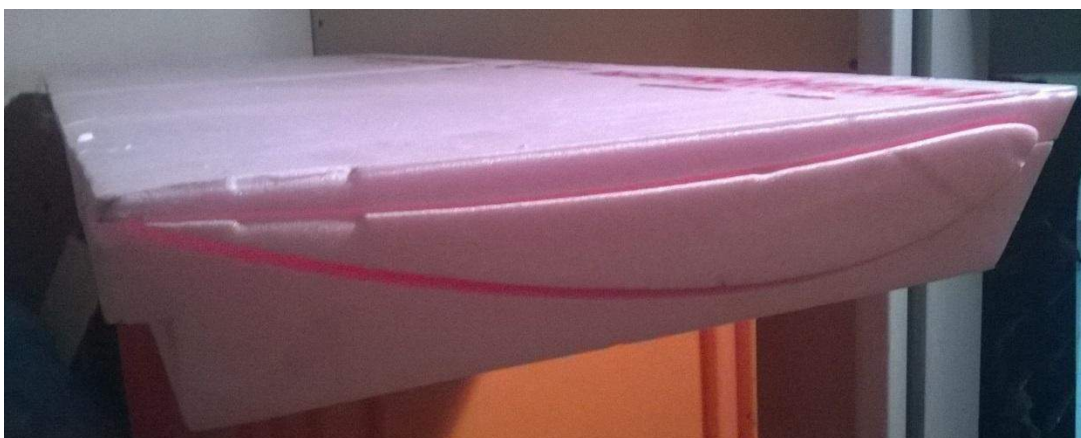
Figure 141: Foam moulds with foam core
