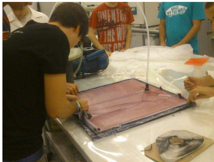
Figure 83: Preparations for the vacuum infusion
