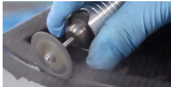
Figure 159: Cutting with Dremel
