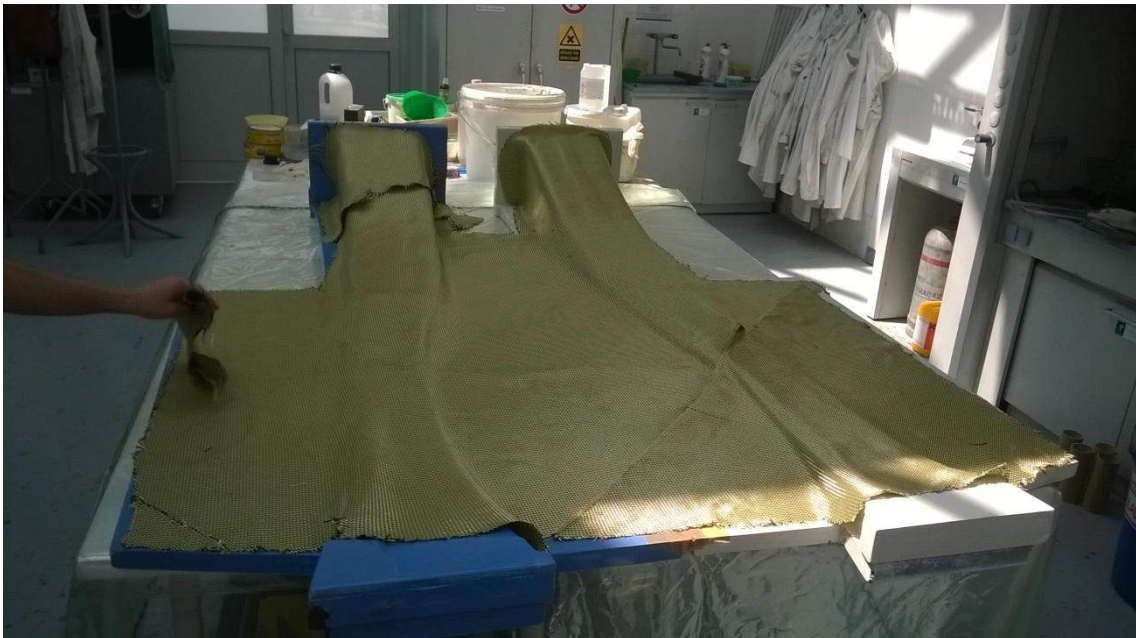
Figure 146: Aramid-Carbon fibre layer created of several pieces
