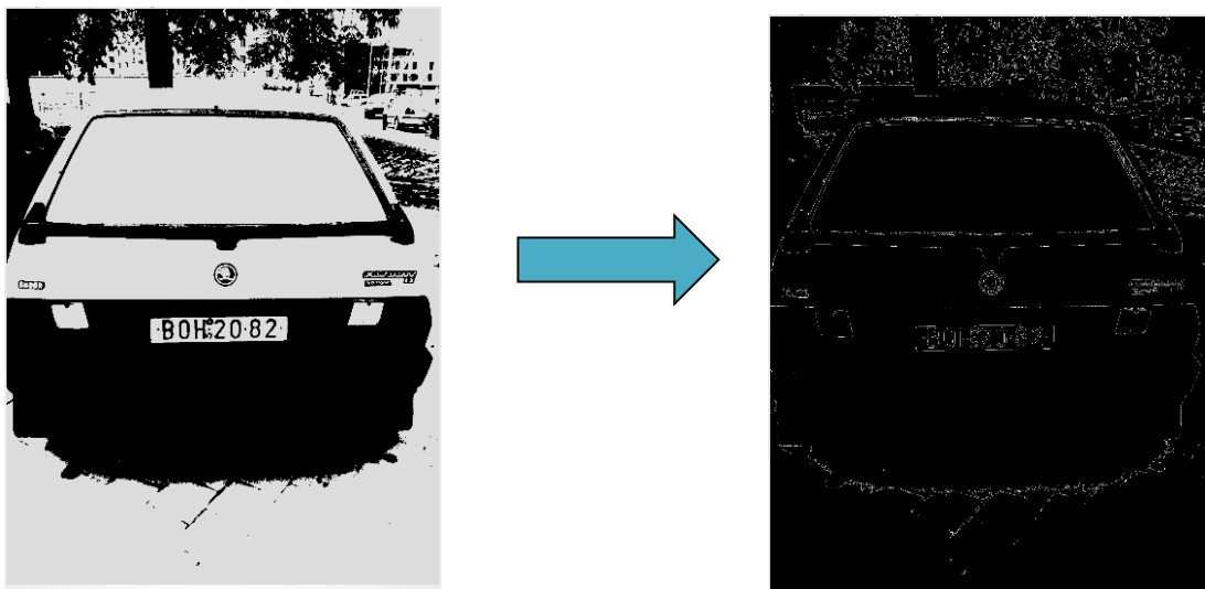
Figure 4.4: Applying Canny algorithm
