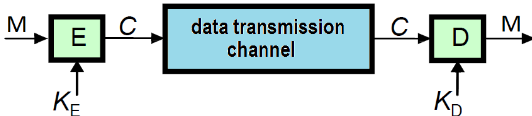
Figure 7.1: Block diagram of the cryptosystem for message confidentiality
