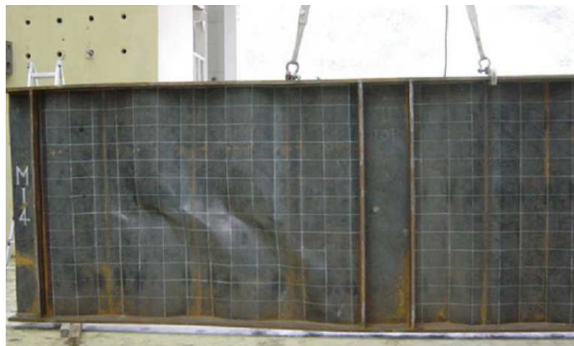
Fig. 23: Moon's specimen after shear buckling failure [47].
