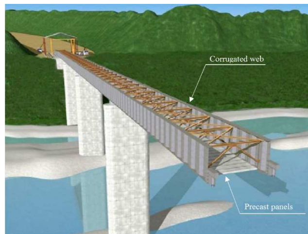
Fig. 7: Incrementally launched superstructure with steel corrugated web.
