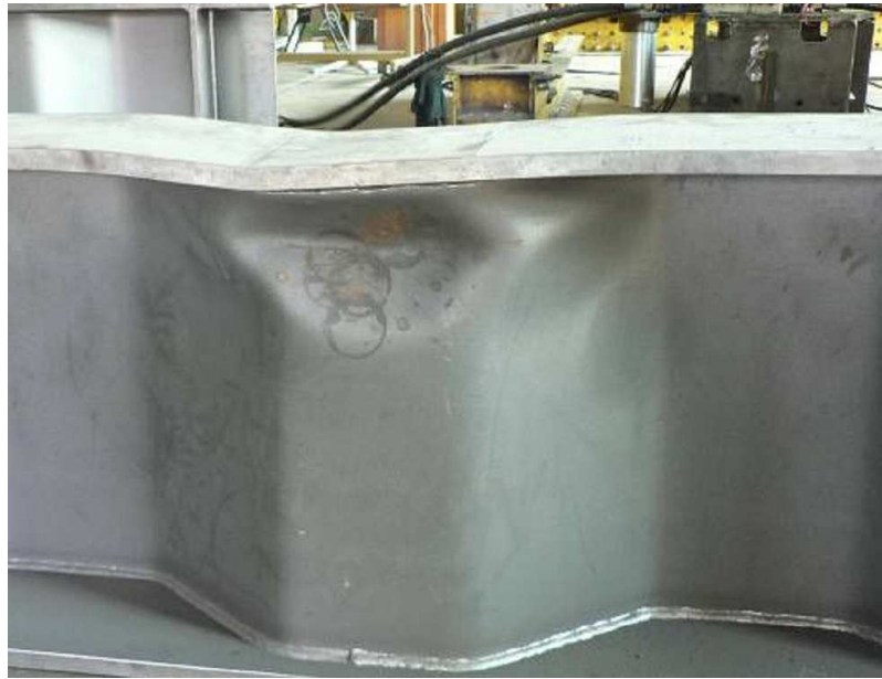
Fig. 25: Local web buckling of Kövesdi's specimen [20].
