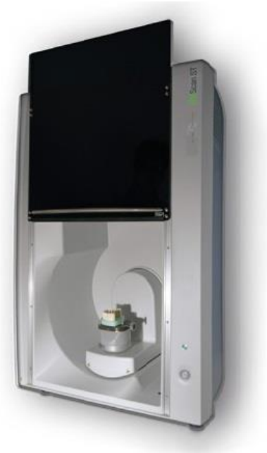
10. ábra: 3D scanner Steinbichler Scan ST {10}
