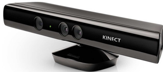
4. ábra Kinect 3D scanner
