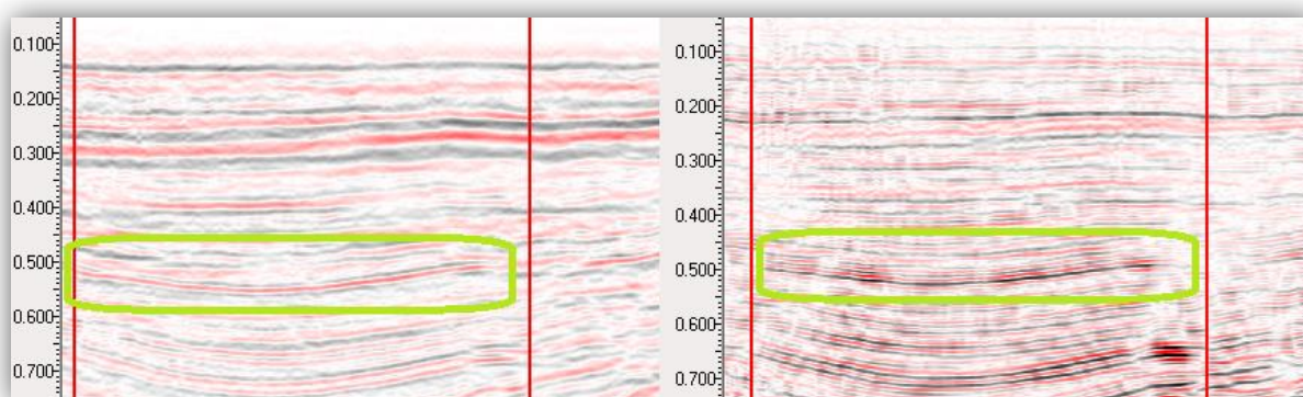
12. Figure: Two time sections about the A-1 line with (left side) and without (right side) automatic gain controlling (The original one is on the left side while the reprocessed one by the Tricon is on the right side)
