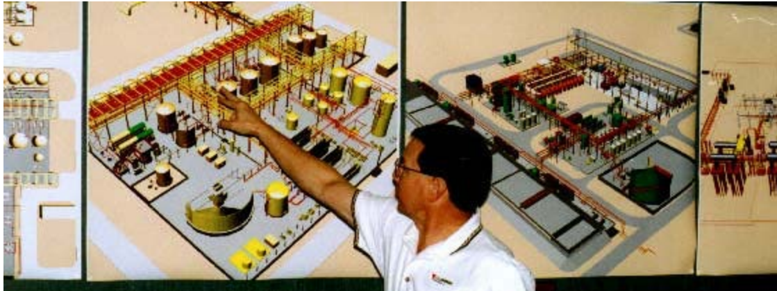
Fig. 22: CalEnergy Vice President of Operation, Jim Turner introduces the new mineral recovery plant, which includes an ion exchange and solvent extraction plant (right), and an electrowinning facility (left) in 1999 (Clutter, 1999)
