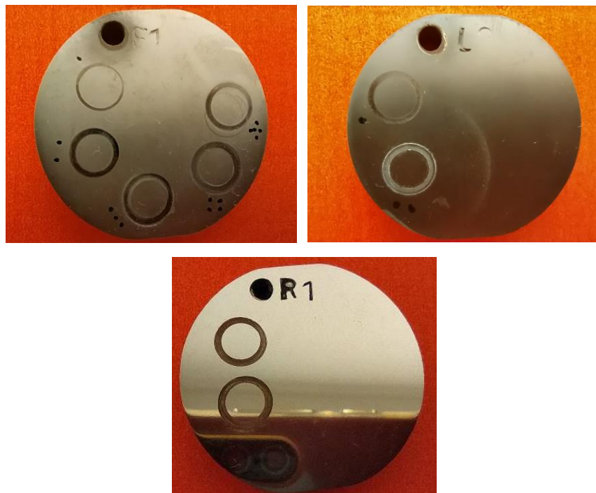
Fig. 31. Coated samples (Formera: top left, Lumena: top right) and the reference material (bottom) with wear tracks
