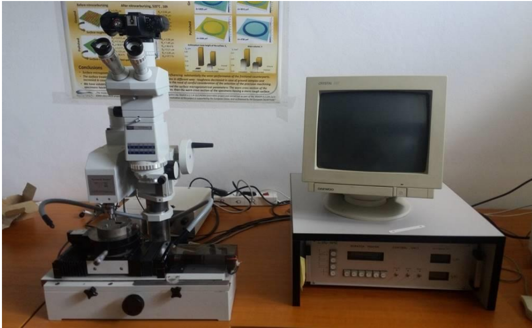
Fig. 21. The SP-15 instrumented scratch tester at the laboratory of IMST, UM
