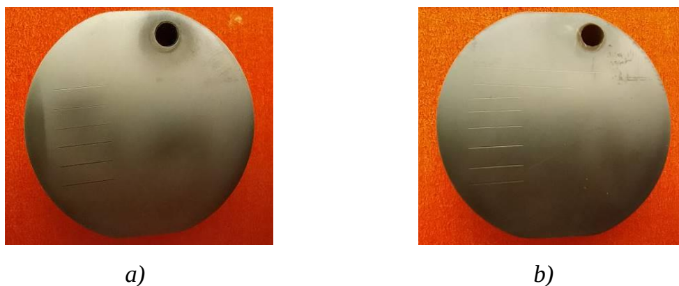
Fig. 26. The photos of coated sample Formera (a) and Lumena (b) with constant load scratches.
