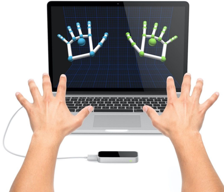
1.8 image Leap Motion Device, the pendrive sized object in front of the laptop [18]
