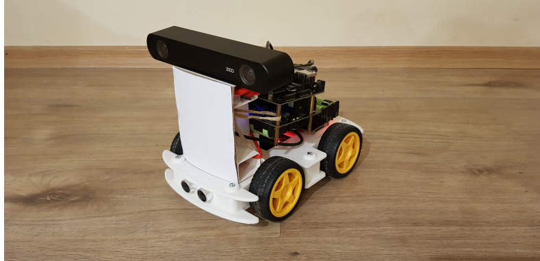
Figure 3: The ground robot used in our real-world experiments. The body is 3D printed and the brain of the agent is given by an embedded computer known as the NVIDIA Jetson Nano. We experimented with multiple cameras, the one visible is the ZED2 [31] stereo camera, but we used the Kinect for Azure camera during experimentation which can be seen in Figure 5.
