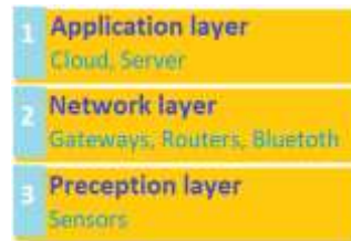
Figure 1. Three layers architecture of IoT
