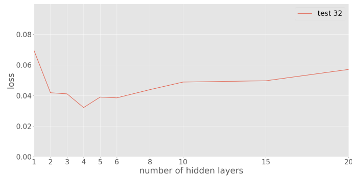
Figure 3.36: Test Performance of best networks of different shapes with 32 width
