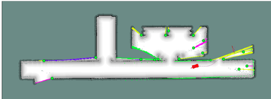
Figure 4.5: Frontier classes visualized with different colours: green - type A (V-shaped) frontier, yellow - type B/I., purple - type B/II., blue - type B/IV. frontiers. There are no instances of turquoise - type B/III. frontiers, as they generally do not appear.
