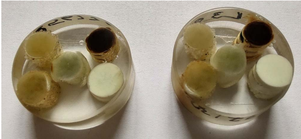
Figure 6 Prepared samples (reference and 30 days aged states, respectively) for SEM analysis
