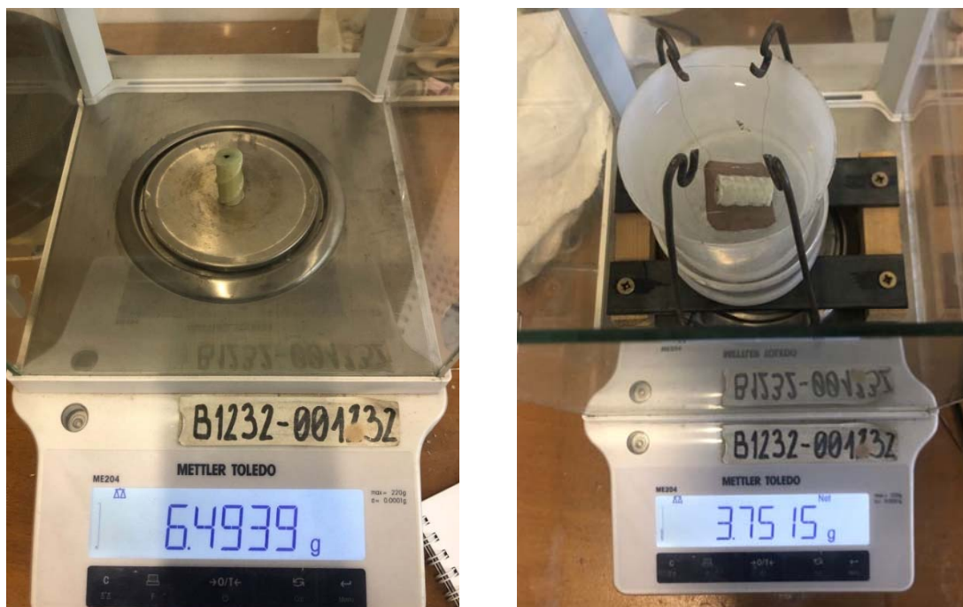
Figure 1 The process of weighting the sample in normal state and while floating in the water
