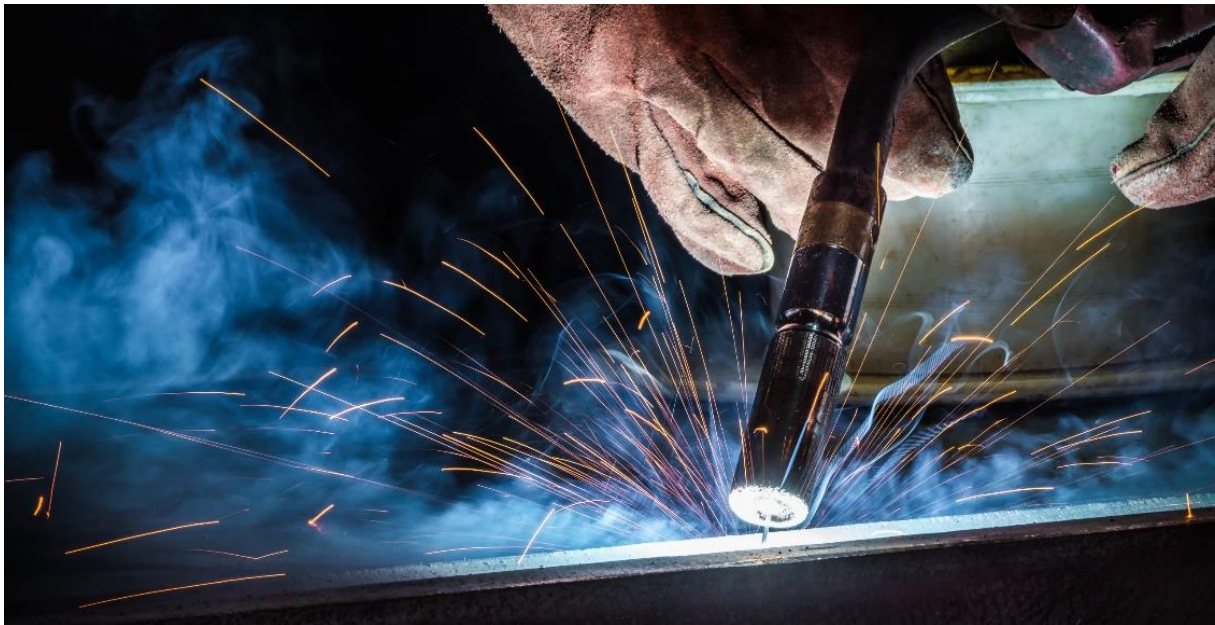
Fig. 7 - MIG/MAG welding during manufacturing [3]
