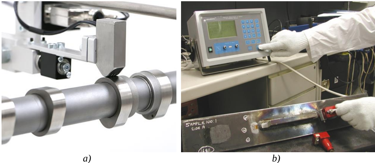
Fig. 14 – a) Barkhausen magnetic noise [11] and b) ultrasonic [15] measurement methods
