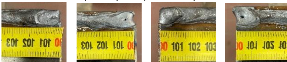
b) Weld pools of RS4-700B specimen
