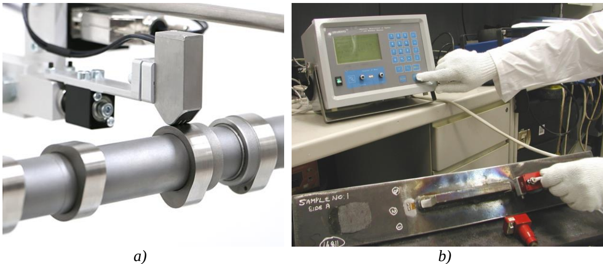
Fig. 18 – a) Barkhausen magnetic noise [15] and b) ultrasonic [19] measurement methods
