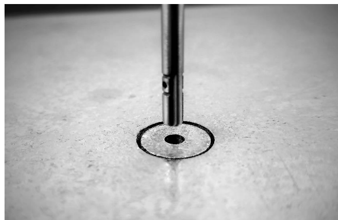
Fig. 13 - Deep hole method [10]
