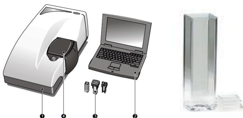
Figure 7. Malvern Zetasizer Nano ZS device and the DTS0012 cell [25],[26].
