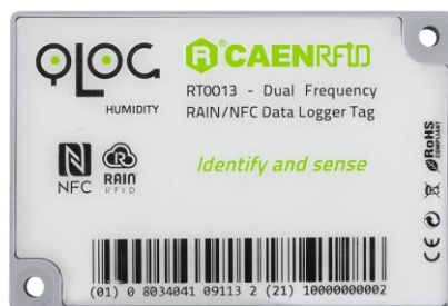
18. ábra: CAEN DFID RT0013- Dual frequency Rain /NFC Data Logger Tag (Internet 2)
