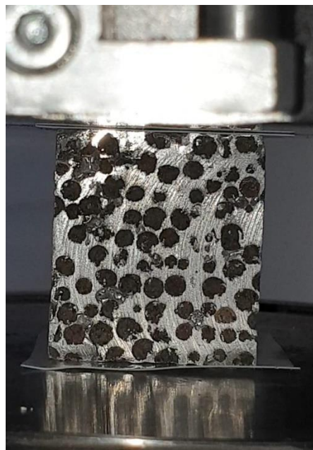
Figure 18. The sample placed in the compression test machine
