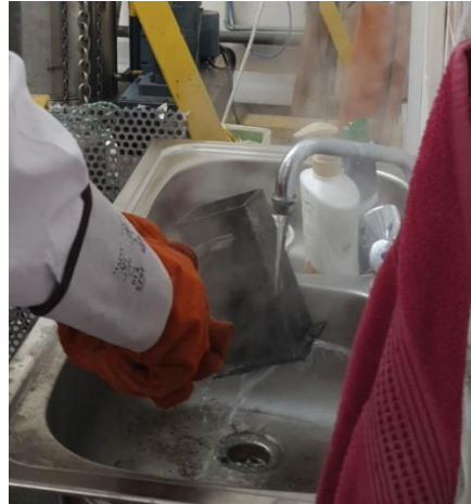
Figure 16. Cold water was poured onto the mould after the infiltration to cool it down
