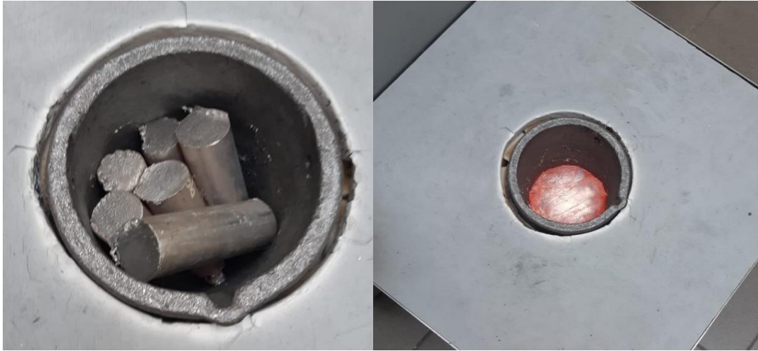
Figure 14. Aluminium being melted in a pot
