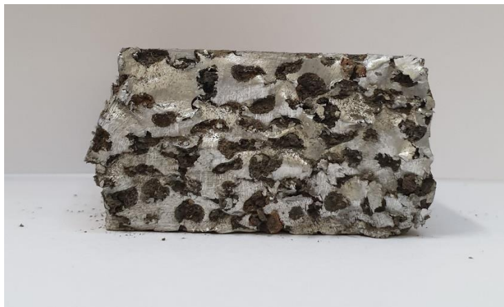
Figure 20. Compressed material after compression test
