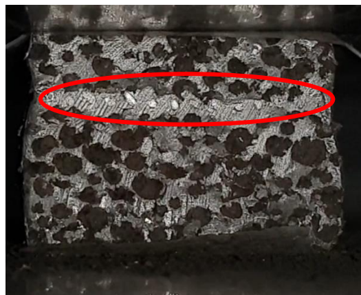
Figure 25. Sample with horizontally located steel grid
