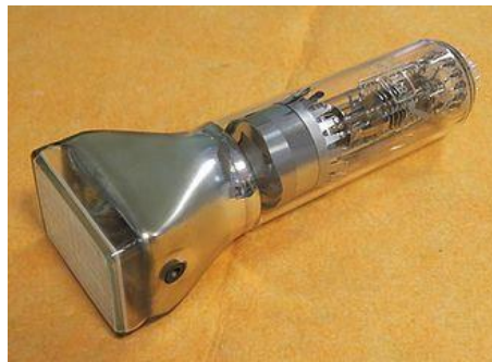
Figure 1. Cathode ray tube found in an oscilloscope
